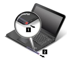
The Tablet Digitizer Pen consists of a tip 2 and a click button 3. Hold the pen and point the tip at the display to move the pointer 1.
